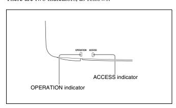
OPERATION indicator: Lights when the on/standby switch on the control panel is in the on (1) position.
